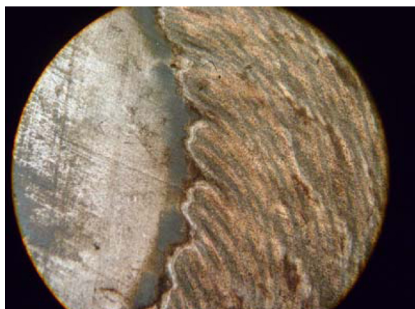
FIG. 6. Optical microscope image of a part of the metallized tracks.
